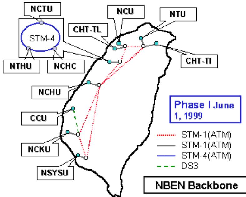
Fig. 10. Topology of NBEN backbone.
