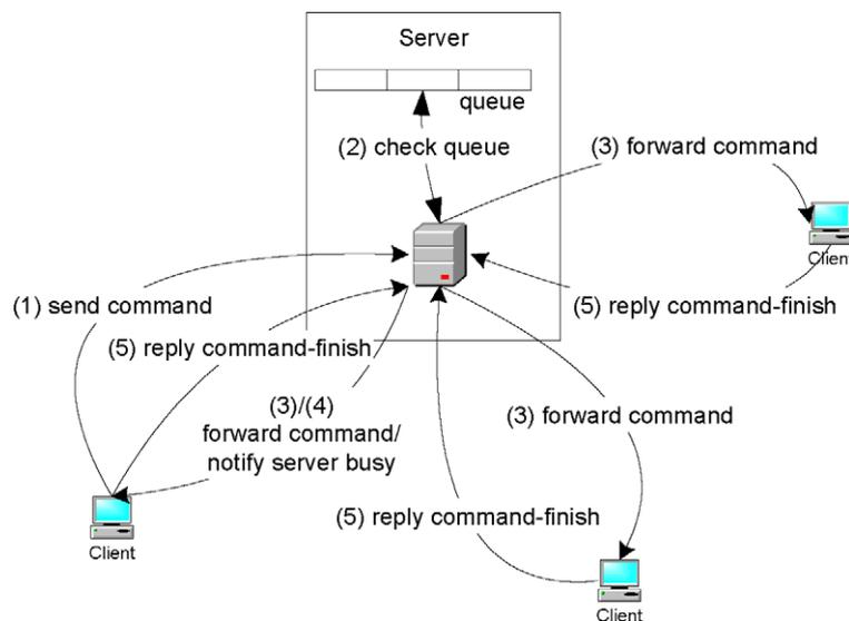
Fig. 4. Command dispatch flow.
