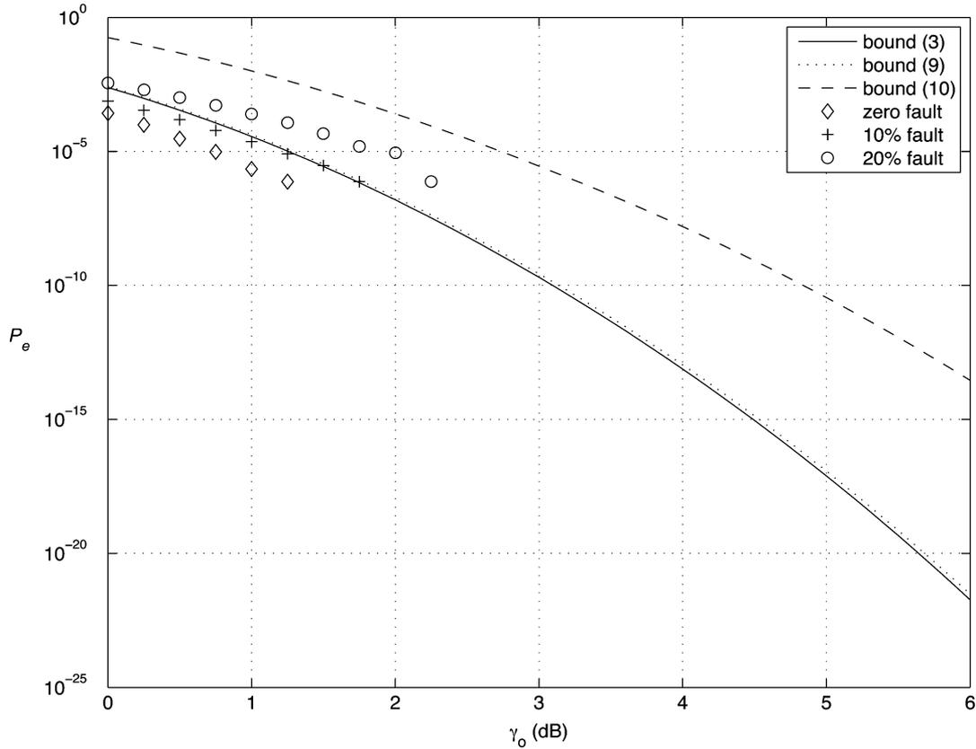
Fig. 6. Simulated performances and performance bounds of the  $8 \times 600$  code that minimizes (9) subject to 10% sensor fault ratio at  $\gamma_s = 0$  dB. The code search is performed for  $\gamma_s = 0$  dB and  $\gamma_o = 6$  dB. The type of the simulated sensor fault is stuck-at-one.
