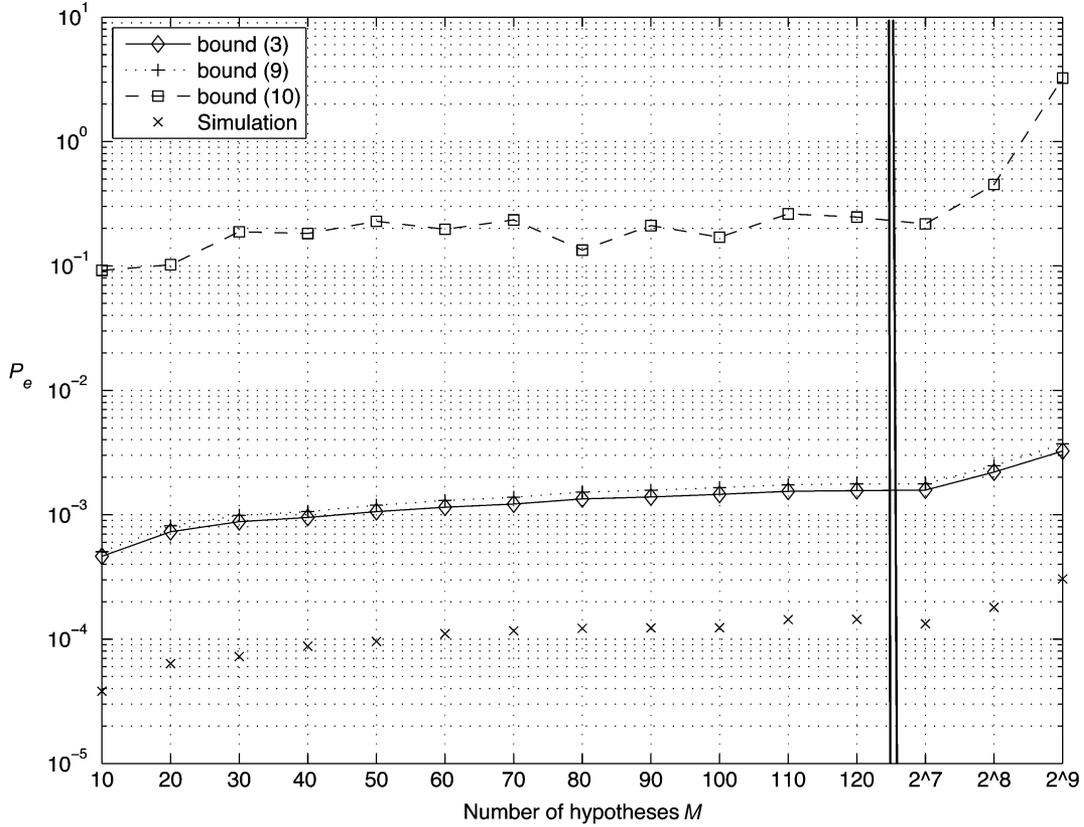
Fig. 14. Simulated performances and performance bounds for the family of best codes that minimize (9). The code search is performed at  $N = 100$ ,  $\gamma_s = 0$  dB, and  $\gamma_o = 6$  dB.
