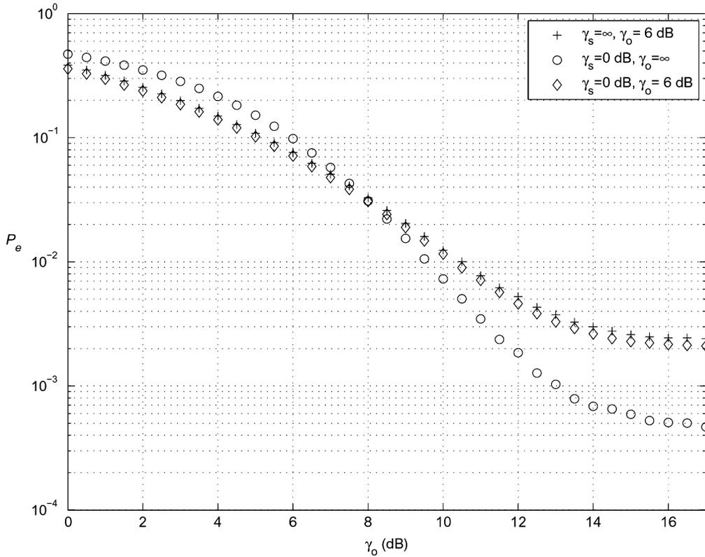
Fig. 4. Simulated performances of three  $8 \times 20$  codes that minimize (9) without the minimum  $d_{\min}$  constraint. The code search for these three codes are, respectively, performed at  $(\gamma_s, \gamma_o) = (\infty, 6 \text{ dB})$ ,  $(0 \text{ dB}, \infty)$  and  $(0 \text{ dB}, 6 \text{ dB})$ . The error probabilities in this figure are simulated at  $\gamma_s = 0 \text{ dB}$ .
