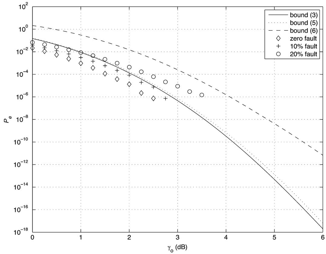
Fig. 11. Simulated performances and performance bounds of the  $8 \times 600$  code that minimizes (5) subject to 10% sensor fault ratio at  $\gamma_s = 0$  dB. The code search is performed at  $\gamma_s = 0$  dB and  $\gamma_o = 8$  dB. The type of the simulated sensor fault is stuck-at-one.
