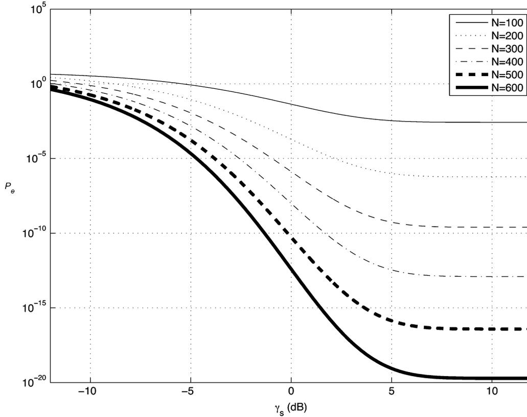
Fig. 2. Bound (10) for the codes listed in Table I (see Section VI-C) at  $\gamma_o = 6$  dB, where we assume that the local observation  $y_j$  is Gaussian distributed with mean  $\ell$  and variance  $1/\gamma_o$  given hypothesis  $H_\ell$  is true.
