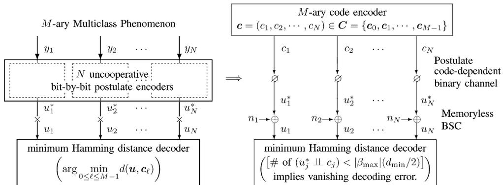
Fig. 15. Equivalent serial-connected binary channel model specifically for wireless sensor networks. The channel noise  $\{n_j\}_{j=1}^N$  for memoryless BSC is independent and identically distributed with  $\Pr\{n_j = 1\} = \epsilon$ . The transition probability  $\Pr\{u_j^* | c_j\}$  is given by (16), and is a function of the codebook  $\mathcal{C}$ .
