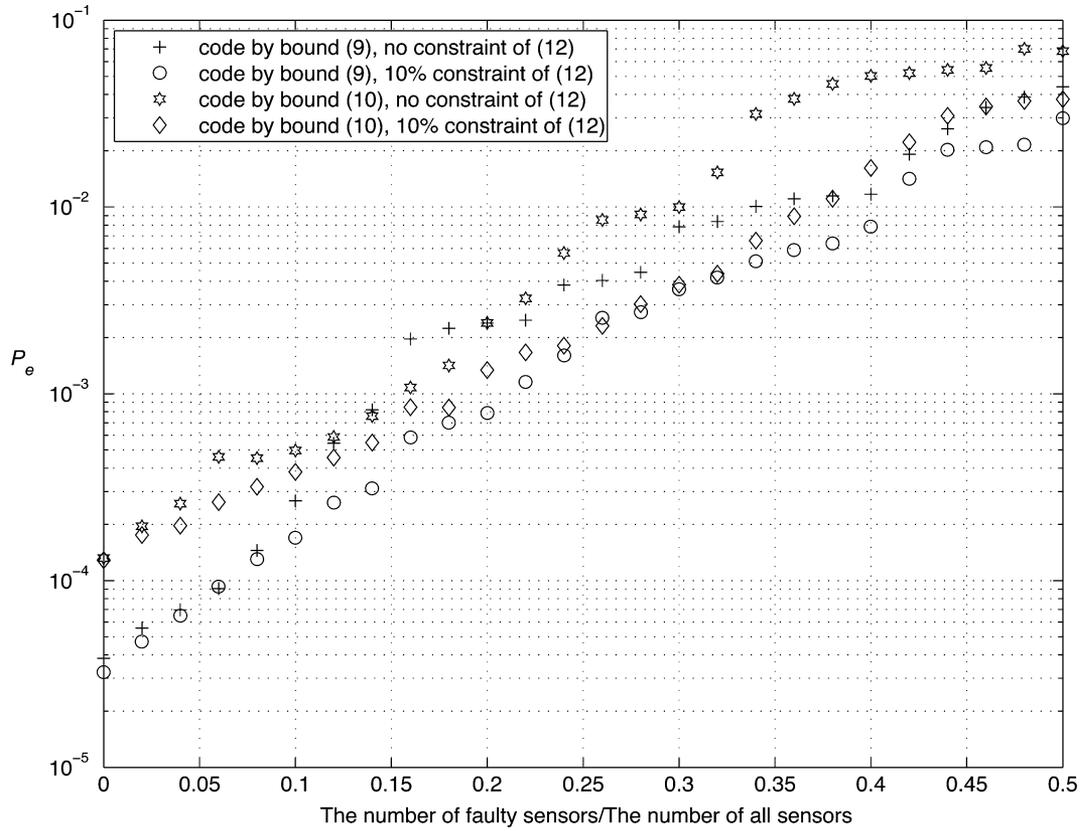
Fig. 8. Simulated performances of four  $8 \times 100$  codes that minimizes bound (9), (10), (9) subject to 10% sensor fault ratio and bound (10) subject to 10% sensor fault ratio. The code search is performed at  $\gamma_s = 0$  dB and  $\gamma_o = 6$  dB. The type of the simulated sensor fault is stuck-at-one.
