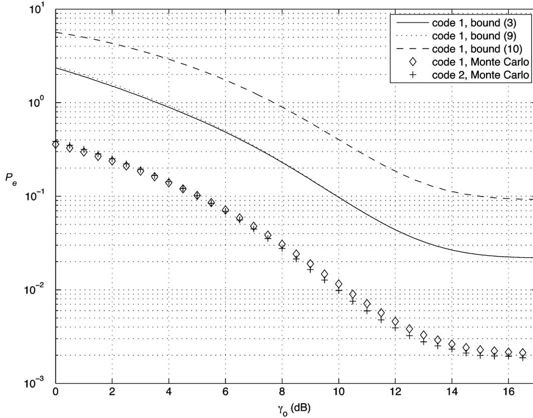
Fig. 5. Simulated performances of the two  $8 \times 20$  codes that respectively minimizes (9) (code 1) and (15) (code 2) at  $\gamma_s = 0$  dB. The code search is performed for  $\gamma_s = 0$  dB and  $\gamma_o = 6$  dB. Performance bounds for code 1 are also illustrated.
