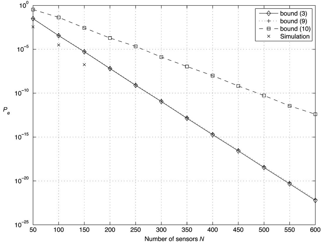
Fig. 13. Simulated performances and performance bounds for the family of best codes that minimize (9). The code search is performed at  $M = 8, \gamma_s = 0$  dB, and  $\gamma_o = 6$  dB.
