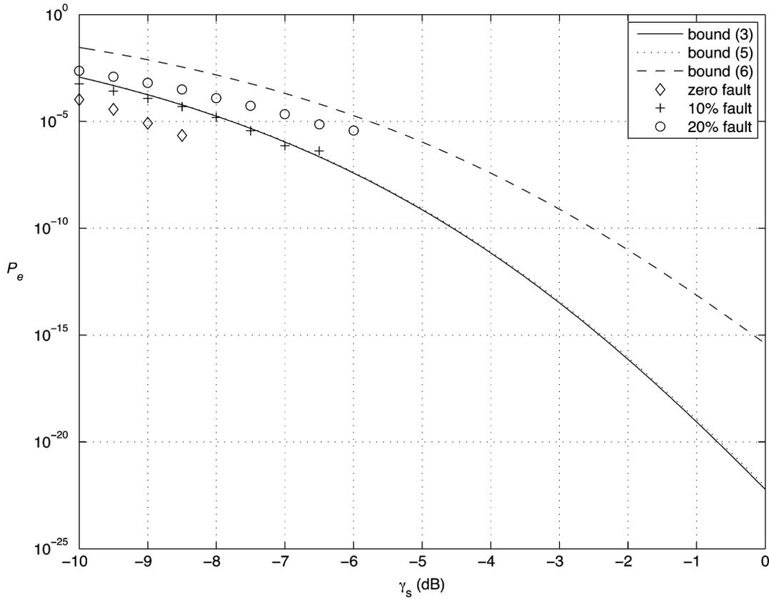
Fig. 10. Simulated performances and performance bounds of the  $8 \times 600$  code that minimizes (5) subject to 10% sensor fault ratio at  $\gamma_o = 6$  dB. The code search is performed at  $\gamma_s = 0$  dB and  $\gamma_o = 6$  dB. The type of the simulated sensor fault is stuck-at-one.
