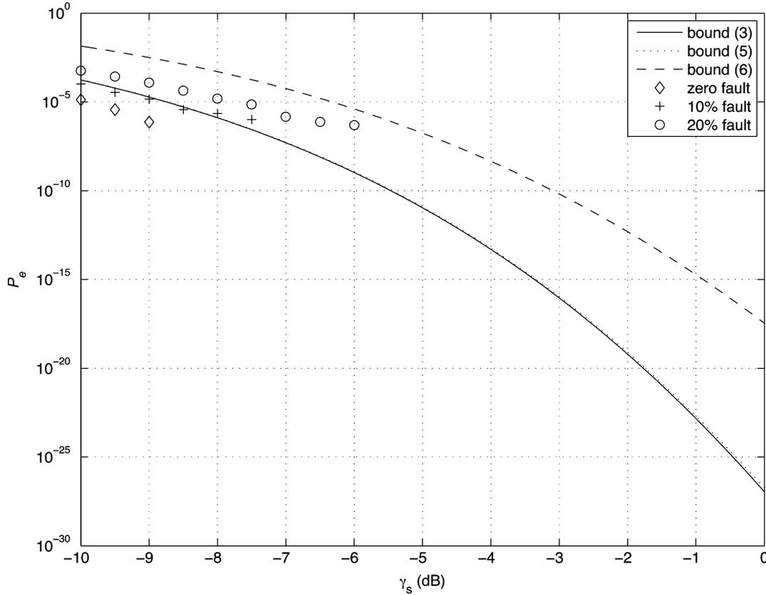
Fig. 12. Simulated performances and performance bounds of the  $8 \times 600$  code that minimizes (5) subject to 10% sensor fault ratio at  $\gamma_o = 8$  dB. The code search is performed at  $\gamma_s = 0$  dB and  $\gamma_o = 8$  dB. The type of the simulated sensor fault is stuck-at-one.
