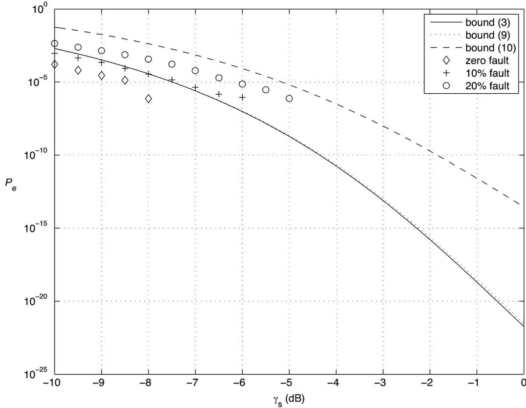
Fig. 7. Simulated performances and performance bounds of the  $8 \times 600$  code that minimizes (9) subject to 10% sensor fault ratio at  $\gamma_o = 6$  dB. The code search is carried out at  $\gamma_s = 0$  dB and  $\gamma_o = 6$  dB. The type of the simulated sensor fault is stuck-at-one.
