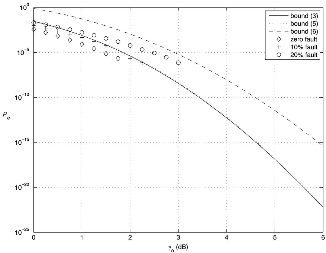
Fig. 9. Simulated performances and performance bounds of the  $8 \times 600$  code that minimizes (5) subject to 10% sensor fault ratio at  $\gamma_s = 0$  dB. The code search is performed at  $\gamma_s = 0$  dB and  $\gamma_o = 6$  dB. The type of the simulated sensor fault is stuck-at-one.
